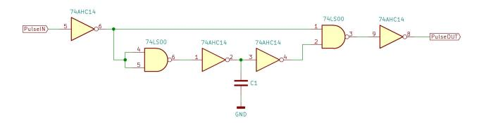
I used the outdated LS chip simply because that is what I had. More modern gates are probably better. The circuit was build on a solderless breadboard making it a bit sensitive to layout details. If you try to built this pulse shaper, be prepared to experiment and to monitor the results with an oscilloscope. Power lines must be decoupled close to the chips.
